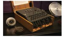
The machines, which steadily became more complex with each iteration, consisted of a series of rotors that, by themselves, encrypted messages input via the attached typewriter. Each rotor performed a simple substitution cipher, but when run through multiple rotors, the encryption reached a staggering level of complexity.
